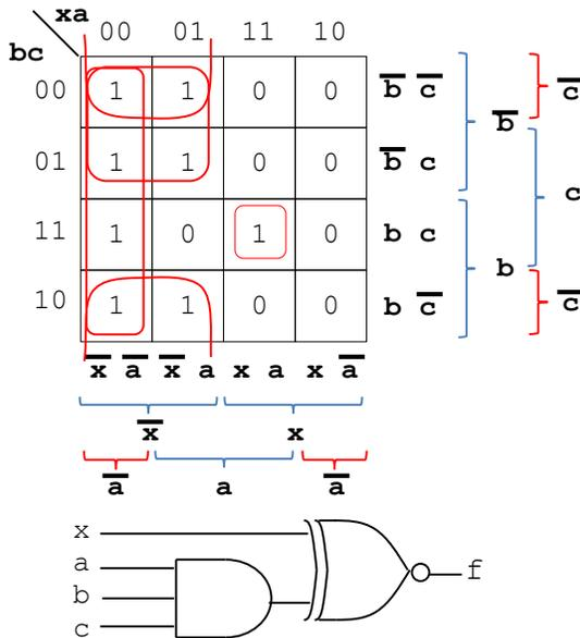
$$f = \bar{b}\bar{x} + \bar{x}\bar{c} + \bar{x}\bar{a} + xabc$$
