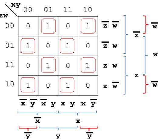
$$f = \bar{x}\bar{y}\bar{z}w + \bar{x}\bar{y}z\bar{w} + \bar{x}y\bar{z}\bar{w} + \bar{x}yzw + xy\bar{z}w + xyz\bar{w} + x\bar{y}\bar{z}w + x\bar{y}z\bar{w} + x\bar{y}zw$$
