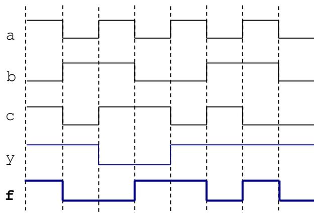
b) The following is the timing diagram of a logic circuit with 3 inputs. Sketch the logic circuit that generates this waveform. Then, complete the VHDL code. (10 pts)
