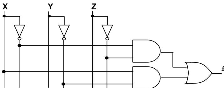
✓  $F = \overline{(\overline{X} + \overline{Z})Y} + X\overline{Y}Z = \overline{(\overline{X} + \overline{Z})Y} \cdot \overline{X\overline{Y}Z} = (X + \overline{Y} + Z)(\overline{X} + Y + \overline{Z})$
